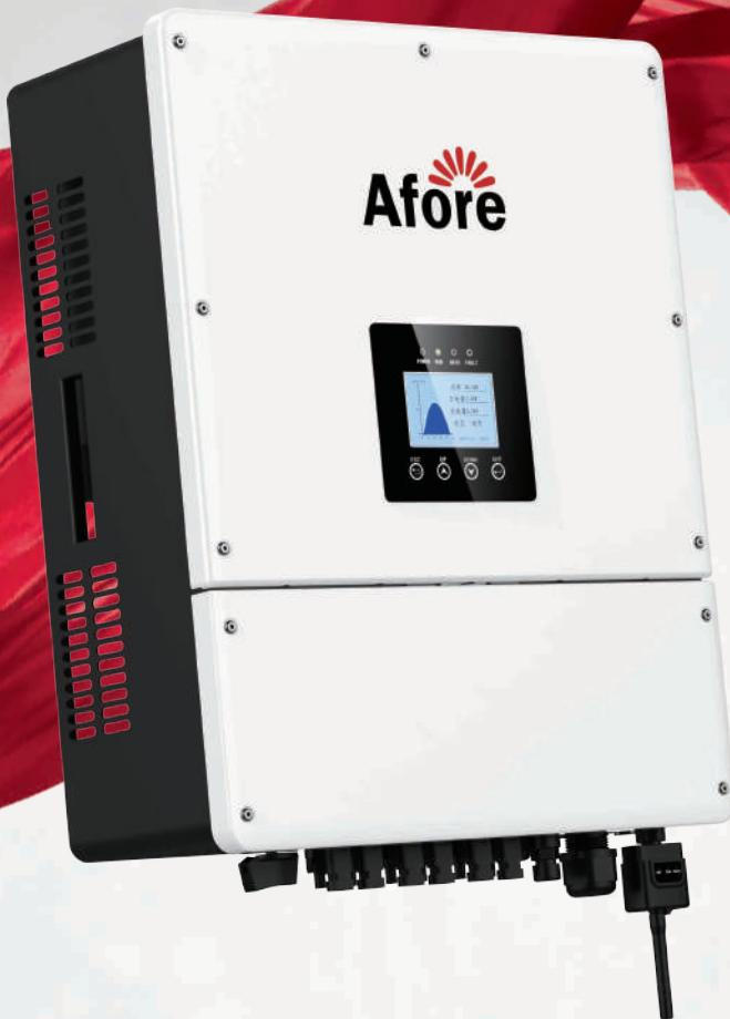
The Afore BNT Series Three-phase string inverters are designed for commercial and power plant PV system applications, rating from 25kW to 40kW. All models with aluminum housings which is anodized, increasing durability and effectively prevents corrosion. Equipped with external inductors, ensure efficient heat dissipation, which significantly improves the reliability and extends the life of the inverters.
